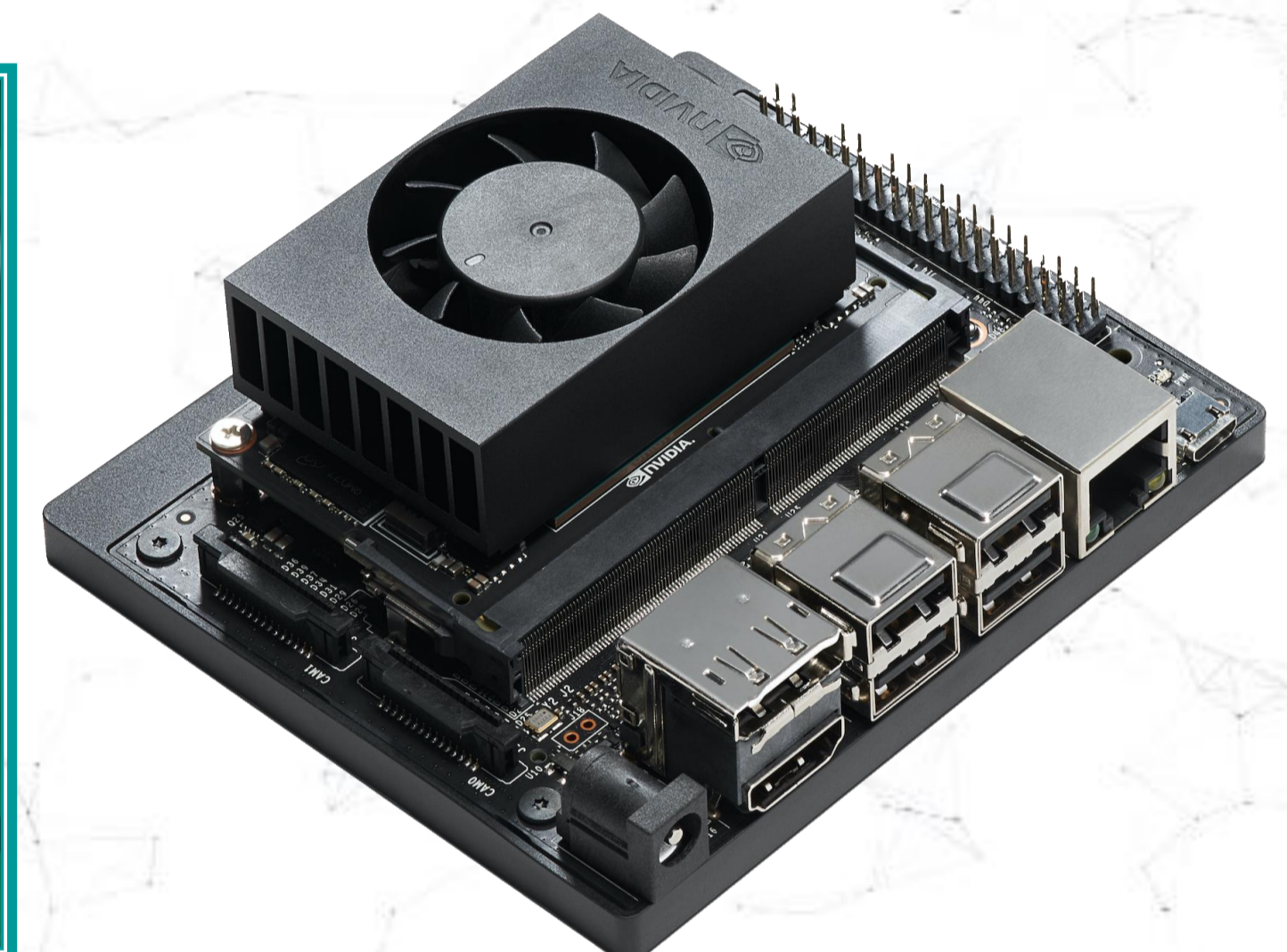
The deep learning accelerator Nvidia Jetson Xavier for real-time classification
