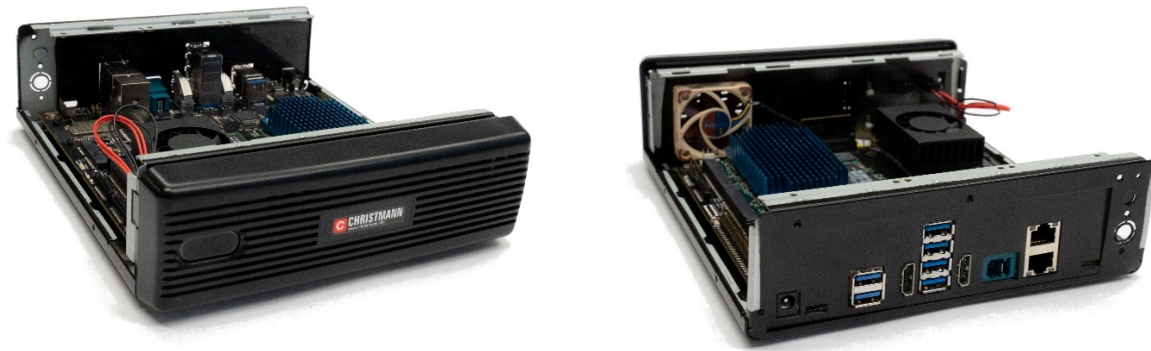
Figure 27 Front and back view of the u.RECS inside Mini-ITX case
