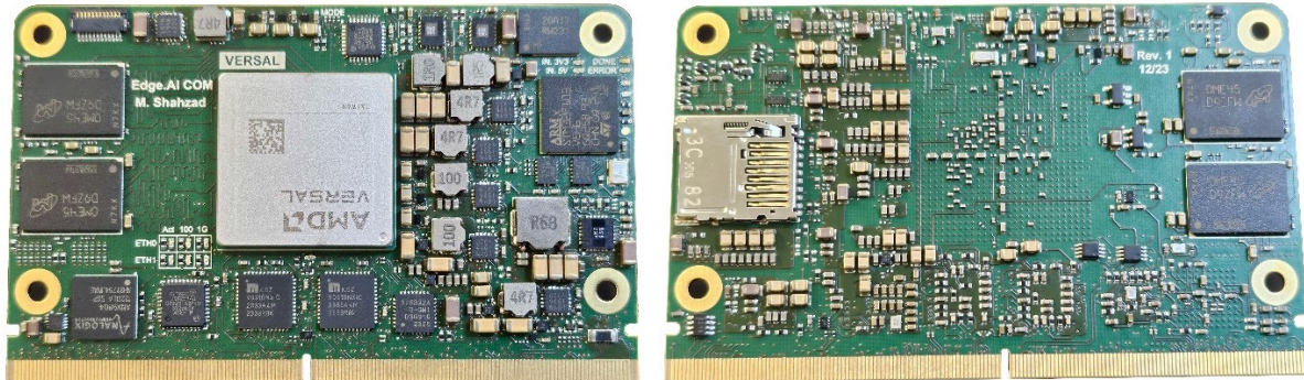
Figure 33: Front- and Backside of the VERSAL Edge.AI COM
