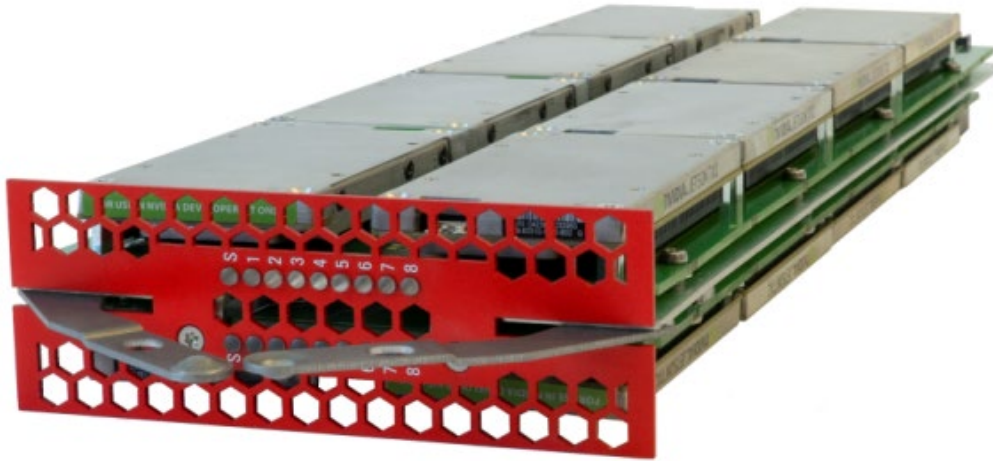
Figure 3: RECS/Box LP Baseboard assembled on mechanical carrier
