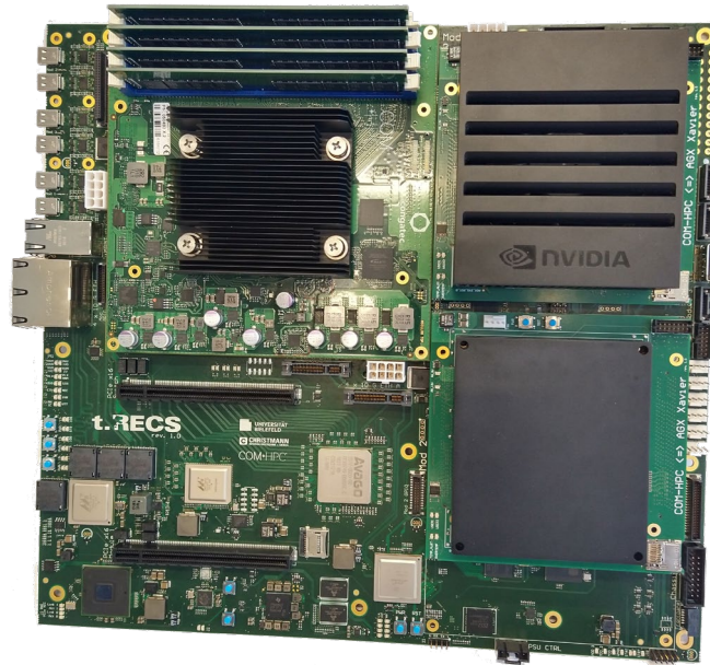
Figure 7: Current revision of the t.RECS PCB with three microservers attached
