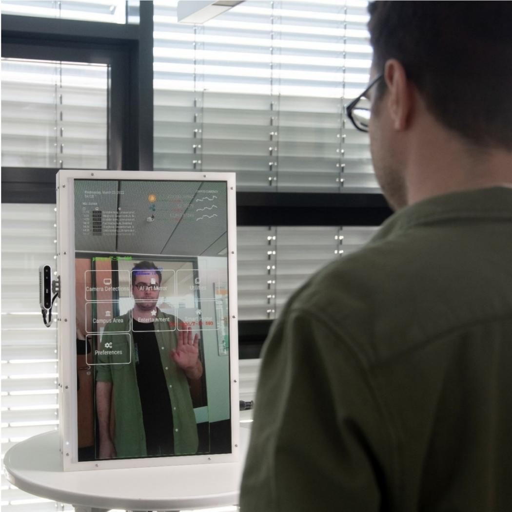
*Figure 30: Smart Mirror prototype utilizing a t.RECS edge server in an acrylic case*
