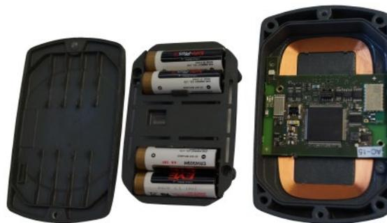
*Figure 2: Smart Field Device for Industrial IoT [source: Siemens]*
