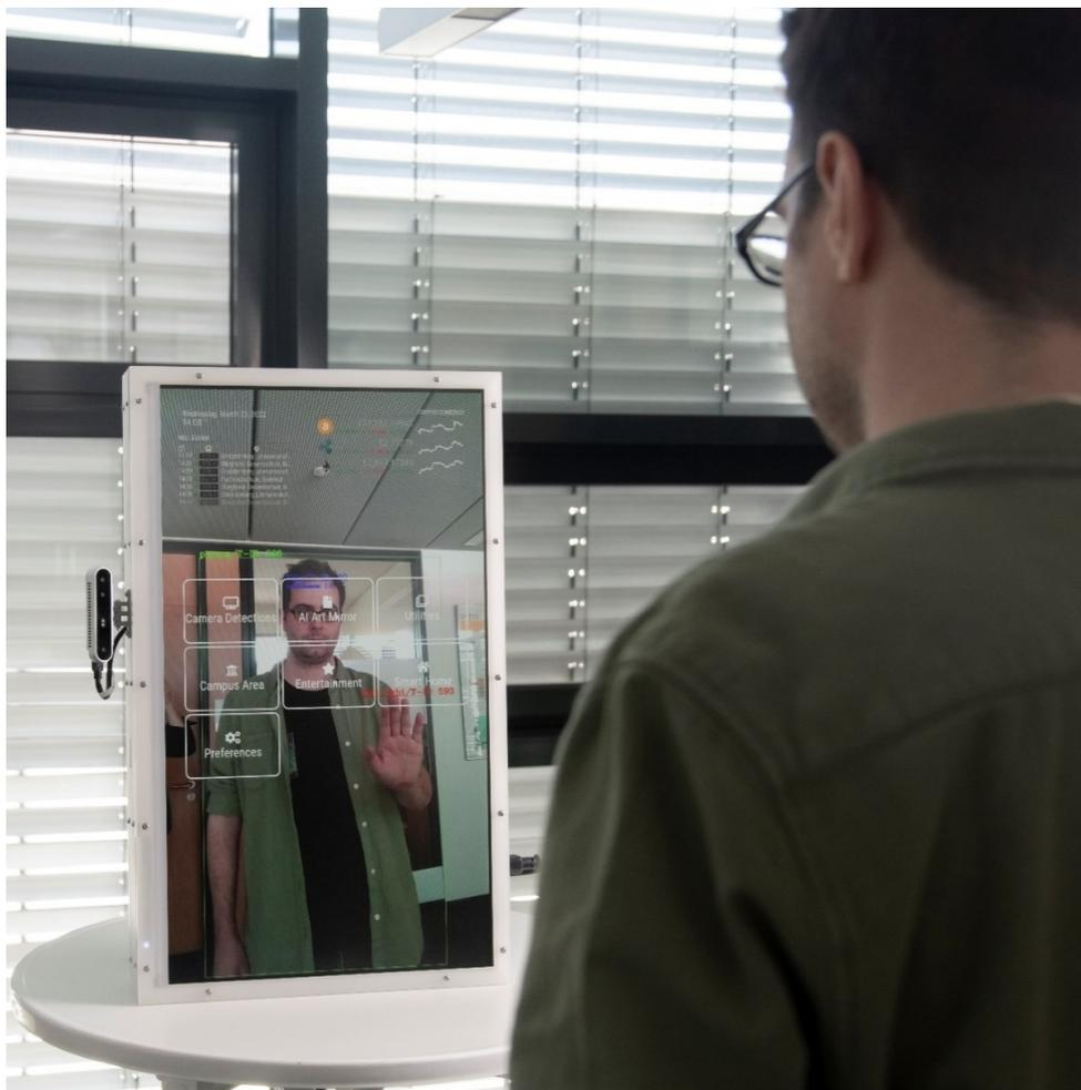
Figure 68: Smart mirror prototype utilizing a t.RECS edge server in an acrylic case
