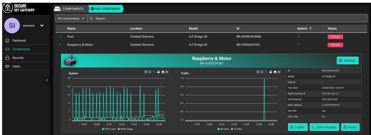
Figure 16: Central monitoring interface for the Secure IoT Gateway
