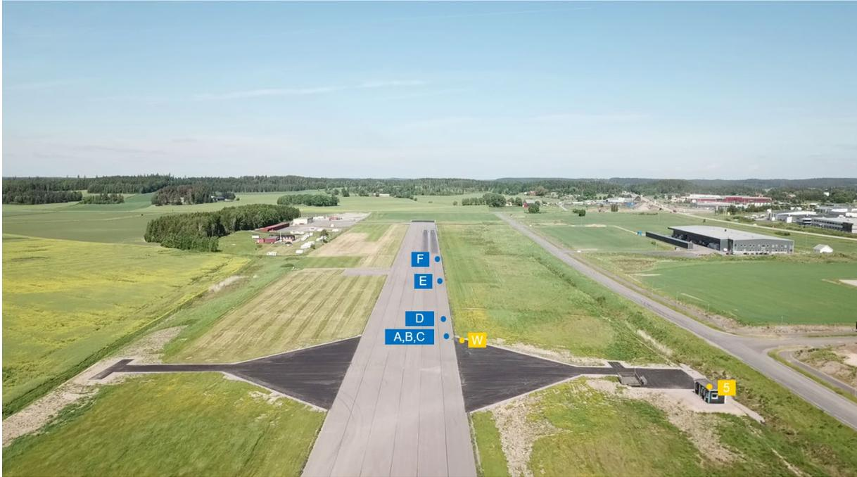
Figure 54: Overview of the positions of relevance during the experiment. Yellow boxes describes positions for the wireless medium and blue boxes describes the positions for the vehicle. A=WiFi Near, B=5G Near, C=Dynamic Start, D=WiFi Medium, E=Dynamic Stop, F=WiFi Far, W=WiFi Antenna, 5=5G Antenna
