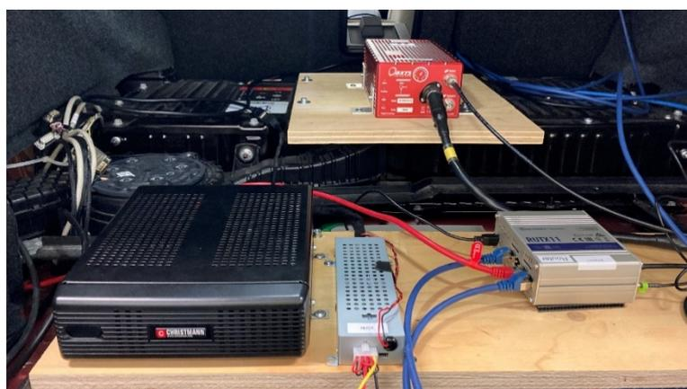
Figure 51: In-vehicle installation of u.recs, OXTS and Wireless Modem
