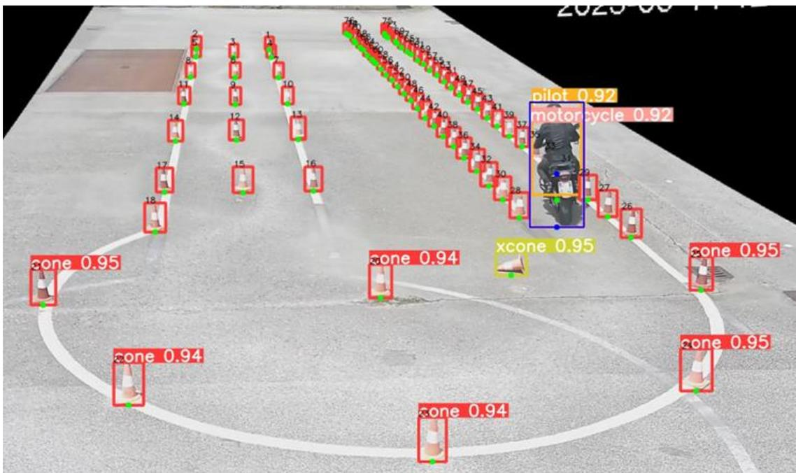
Figure 31 Example of all the class detected with a confidence greater than 92%(xcone represent the fallen cone).
