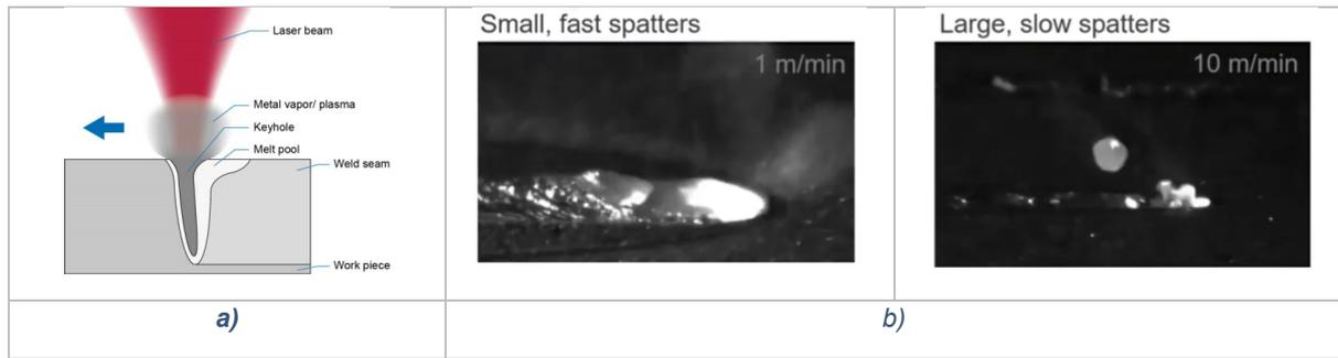
Figure 6: a) Parts and phenomena of a laser-based welding process; b) Different melt-pool dynamics and spatter behavior as a consequence of the keyhole effect.
