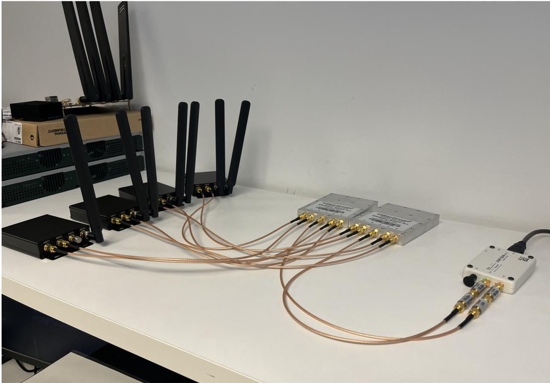
Figure 4.4. Client's 5G modems connected to the basestation
