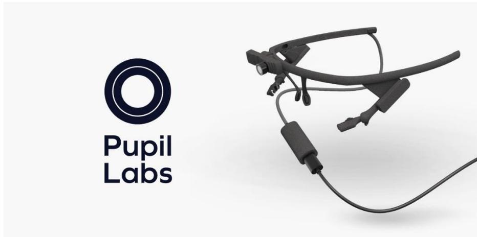
Figure 27 Pupil Labs Core glasses with eye pupil tracking system.
