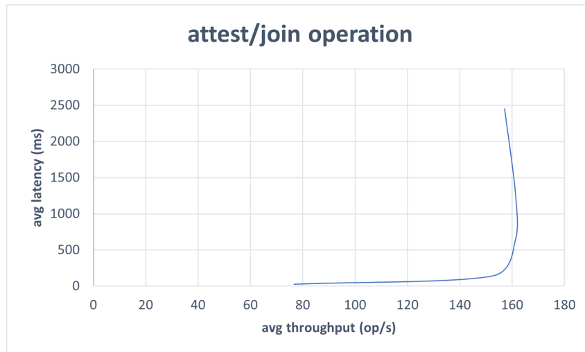
Figure 5.8. Performance evaluation of the attest/join operation, using 11 client machines and a maximum of 6000 clients. The graph presents a relation of throughput and latency in function of an increasing number of simulated devices interacting with the system.
